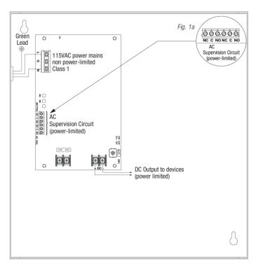
[L] and [N]: This is the primary AC power input terminal and connects to a
